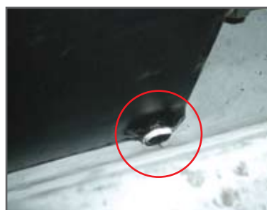
▲ Fuel tank drain point Vidange reservoir carburant
